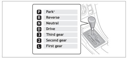
\* The engine switch must be "ON" and the brake pedal depressed to shift from Park.
